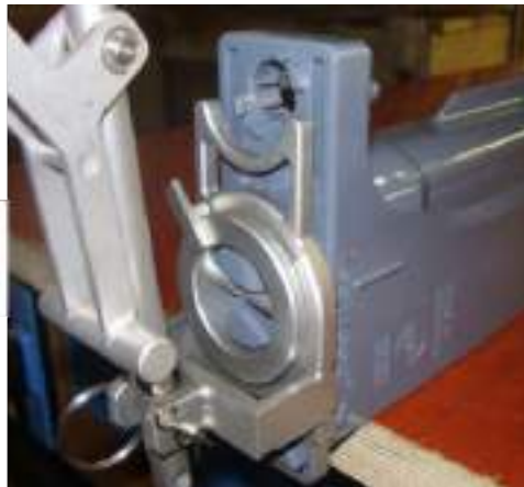
figure 5.35 - fitting faceplate to module
