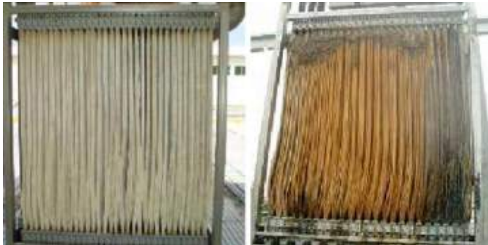
figure 10.3 - acceptable (left) & unacceptable (right) solids accumulation
