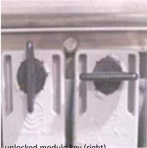
figure 5.34 - unlocked module key (right)
