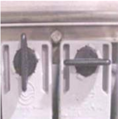
figure 10.5 - locking key locked (left) & unlocked (right)
